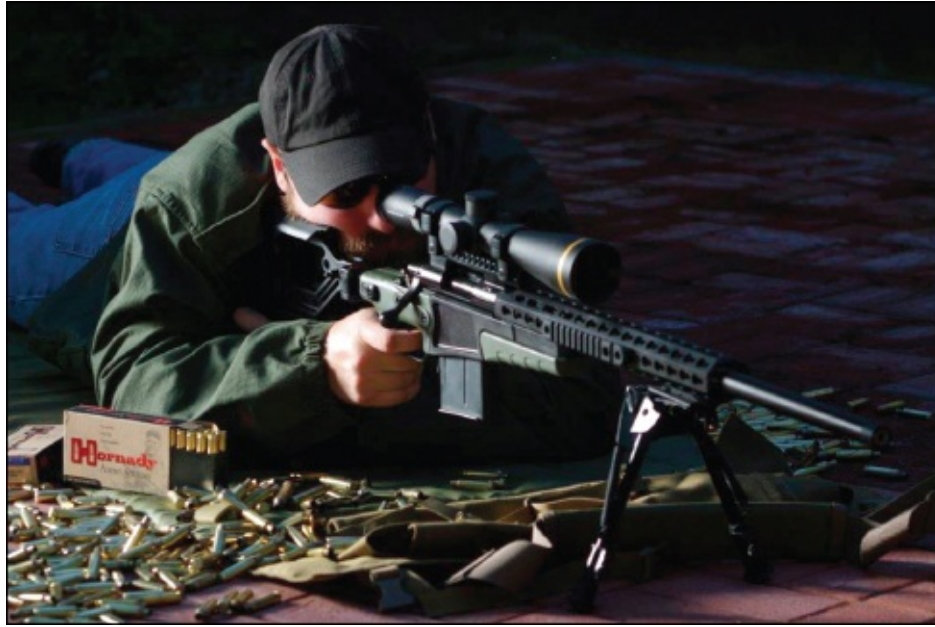
Nathan Towsley shooting a custom-built 6.5 Creedmoor rifle. It has a Stryker Ridge action, Bartlein barrel, and an Accuracy International chassis with an X-Treme Shooting Products trigger and Leupold scope.
