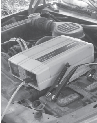
Inverter cables connected to car battery
