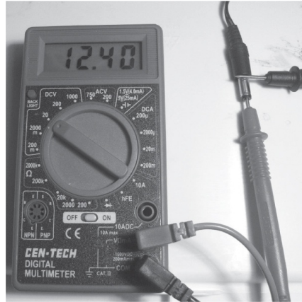
Checking the voltage of the plug
