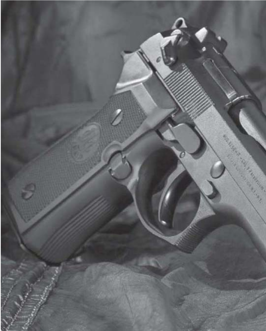
A closeup of the tried and true Beretta Model 92, showing its double-action/single-action trigger and ambidextrous safety system.
