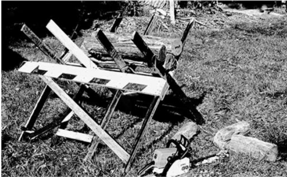
A sawbuck made from salvaged lumber holds 3–7 logs at a time, reducing the number of saw cuts required to produce stovewood. [Credit: Creighton Hofeditz]
