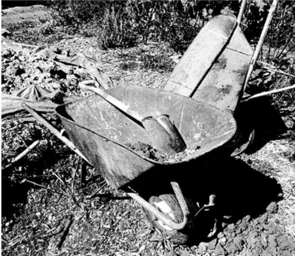
These 13-year-old all-steel wheelbarrows have a narrow profile and a center of gravity over the wheel. The “nose” does not protrude unduly, and the curved front struts will never get caught on rough ground. [Credit: Creighton Hofeditz]
