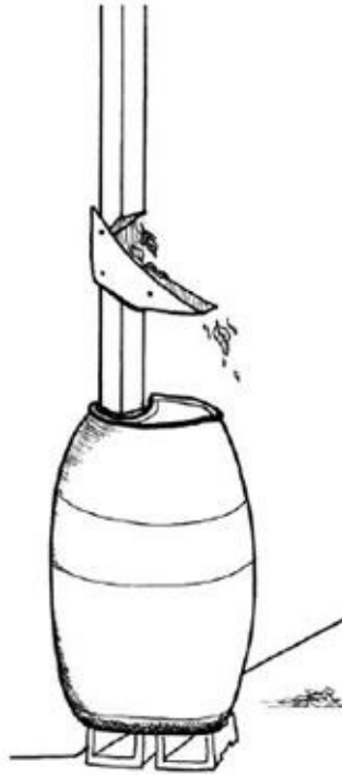
Cutaway downspouts are a commercial item or can be homemade. [Credit: Abi Mustapha]
