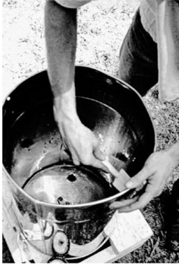
D. A small centrifugal spinner can extract honey from two frames at a time. [Credit: Peter Bane]
