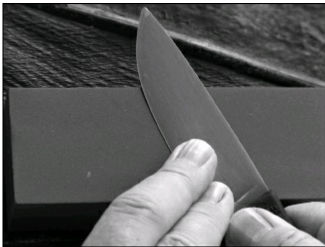
Sharpening Fällkniven F1 with a convex edge by drawing away from the edge.
